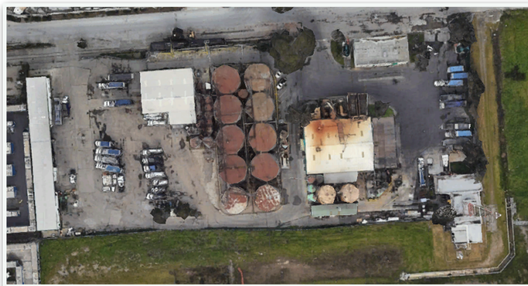
Figure 5. Satellite photo of Darling's San Francisco facility. The brown cylindrical shapes in the center of the photo are 100,000 gallon storage tanks. Source: Google Maps.
